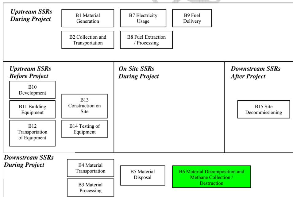
\* Sources, sinks and reservoirs selected for measurement and monitoring under this protocol are highlighted.
