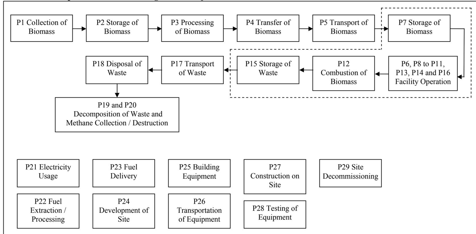
**FIGURE 1.4: Simplified Process Flow Diagram for Baseline Condition**
