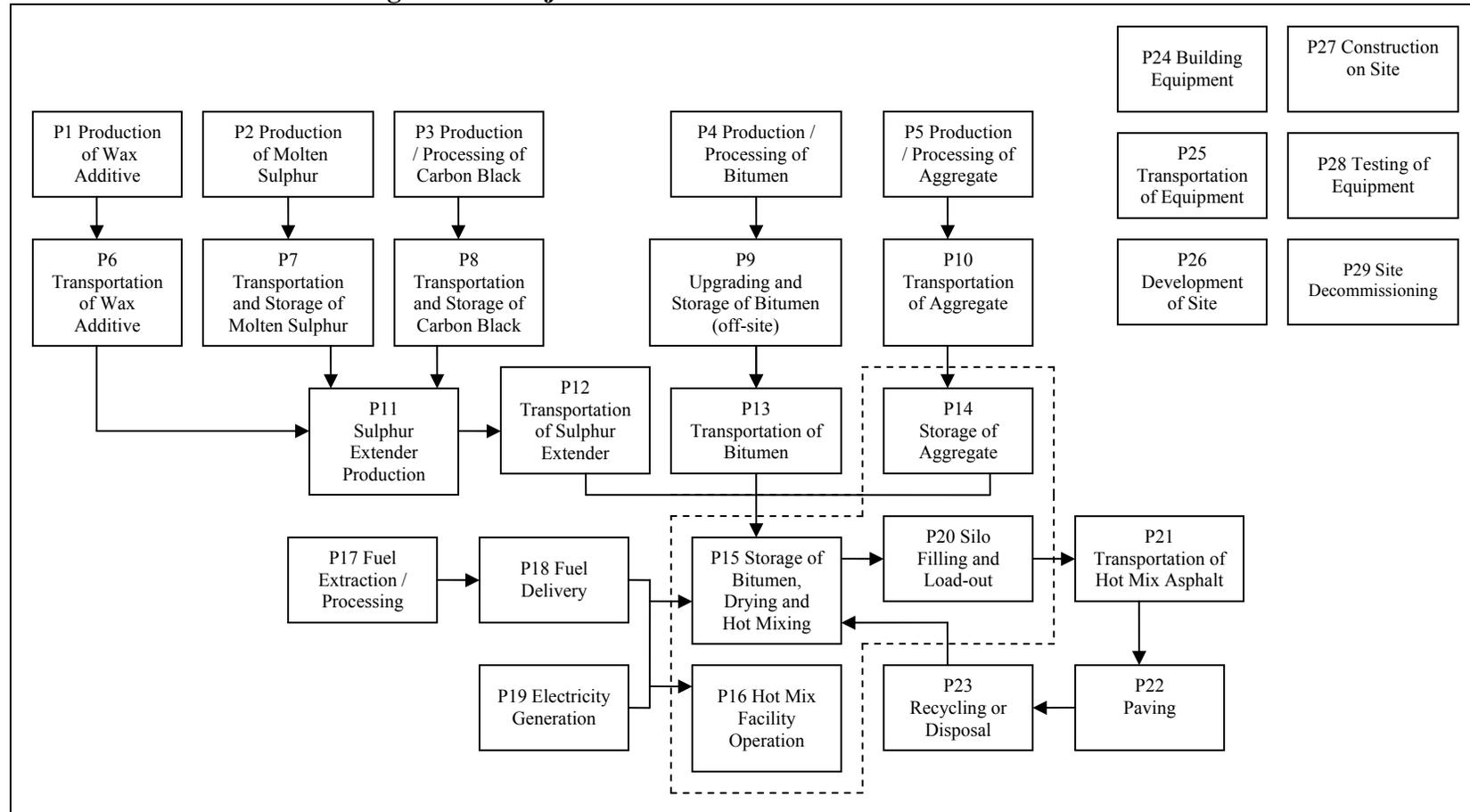
**FIGURE 1.2: Process Flow Diagram for Baseline Condition**
