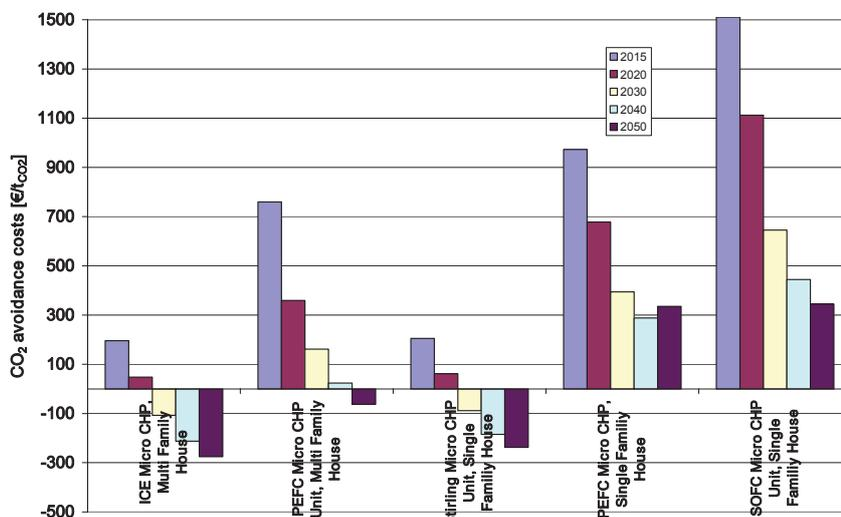
Figure 2 Cost in Euro per tonne of CO<sub>2</sub> abatement using various CHP systems
