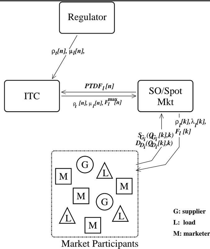
Fig. 5. The information exchange between the market participants and the SO for the allocation of residual transmission capacity in the spot market for energy
