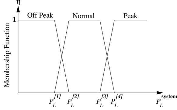
Fig. 7. Membership Functions for Individual Load Pattern
