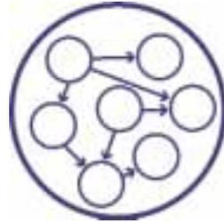
*Above: A DOME module is a mathematical simulation of one element of a complex design, in this case the engine of a vehicle. The smaller circles linked by arrows are interdependent engine components and processes. The enclosing circle represents the DOME "wrapper" which facilitates communication with other modules.*
